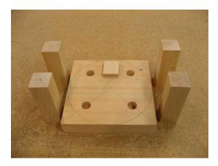
For my part I cut off the corners from the stool top on the band saw to make an approximately round cross-grain blank to avoid chipping the piece when roughing-out to round on the lathe.
